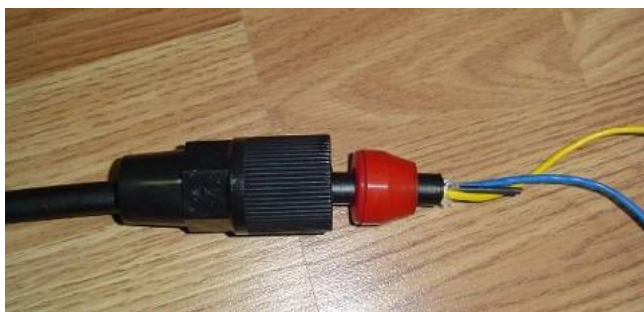
(2) Put bolts and suitable silicon rubber on the stripped cable.
