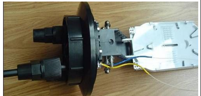
(3) Penetrate the stripped cable to the bracket through the entry ports.
